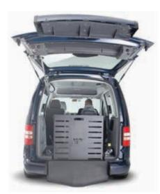
All of our driver solutions have a fully automated tailgate and ramp system, so the car can be used completely independently by the wheelchair driver. To enter and exit the vehicle simply press a button on your key remote or dashboard and the fully automated rear end will open or close.
