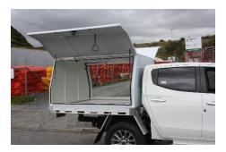
Auto Transform brings you a Box Body which is one of the lightest on the market. Made from 3mm aluminum it sits on an aluminum flat deck tray. This Auto Transform Box Body not only maximizes space but also allows you to save on weight whilst transporting all your equipment. With its modular design, the options for customised fit outs and optimising your specific space are endless. We have Box Bodies for single, extra and double cab.
