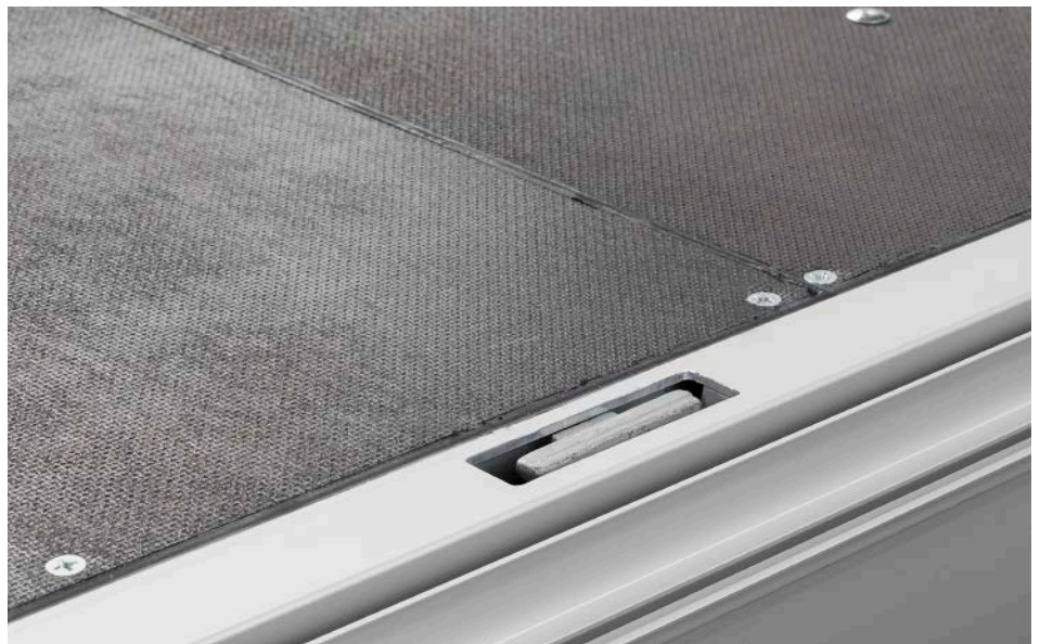
Lashing ring embedded in the floor
