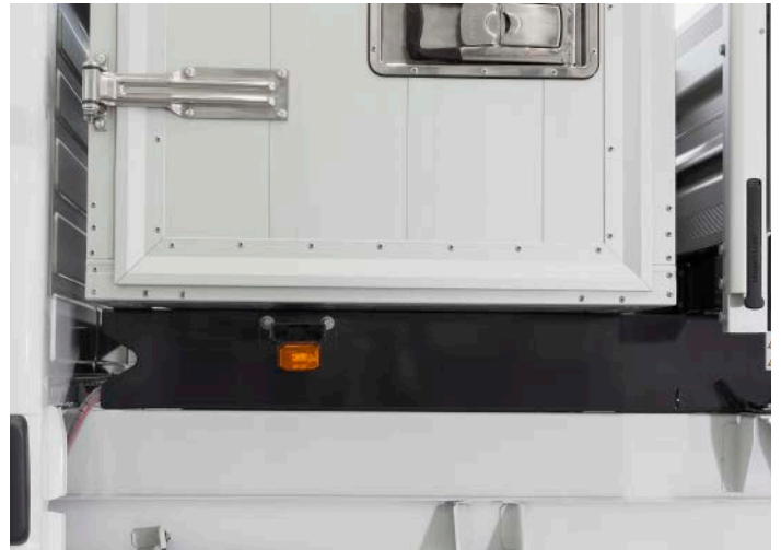
Extension of the subframe for mounting a loading crane or a tool box behind the driver's cab
