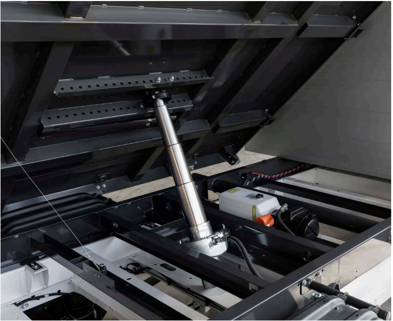
Chassis with tipper platform-lifting cylinder with electro-hydraulic drive
