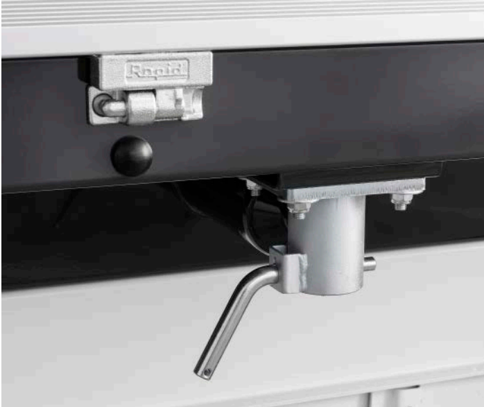
Pin to determin the tipping direction
