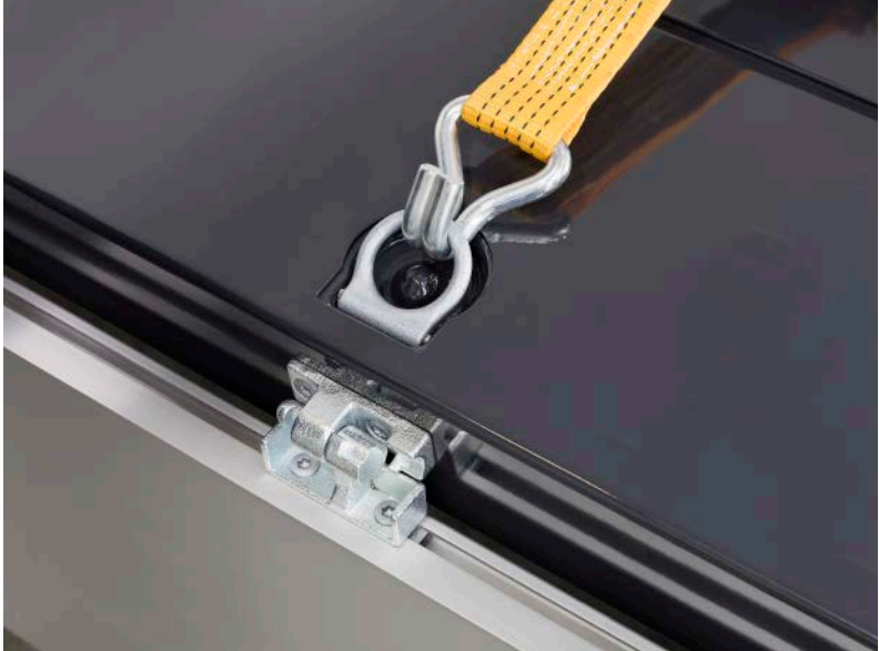
Lashing ring with belt for securing the load
