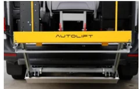
A discreet underfloor hoist designed to maximise interior space while delivering safe, reliable wheelchair access.
