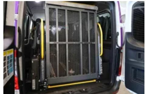
A lightweight, full-platform hoist designed to reduce vehicle load while maintaining strength, safety, and reliability.
