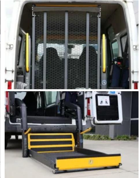
A robust, full-platform hoist designed for larger wheelchairs where stability, simplicity, and reliability are critical.
