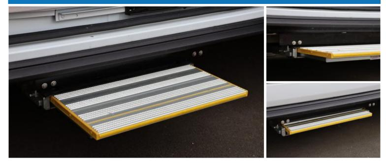
The Step 550mm (21.65) is an automatic operated side step perfectly suited to your passenger transport needs. Making your life easier though our simple and durable step.
