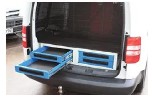
This huge, space saving under-floor drawer unit is safe and secure, preventing theft and movement during transport.
