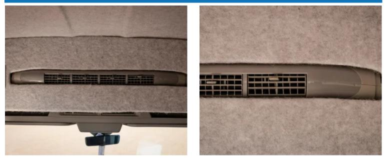
Robust Slimline Air Blower Unit with three-speed fan for heating and cooling.
