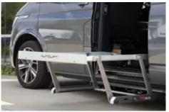
The new multilink F6 hoist has a 300kg maximum lifting capacity to suit all your wheelchair requirements.
