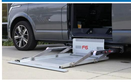
The new multilink F6 hoist has a 300kg maximum lifting capacity to suit all your wheelchair requirements.
